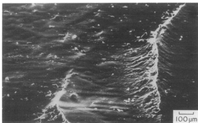
Figure 12 Scanning electron micrograph of short rod fracture surface of PMMA
